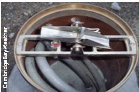
Rain Gauge with tipping bucket structure.
